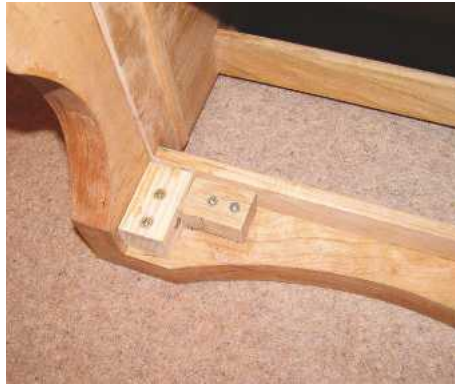
▲ Pic.8 The plinth was attached by screwing through the bottom rails into blocks glued to the inner faces of the plinth
